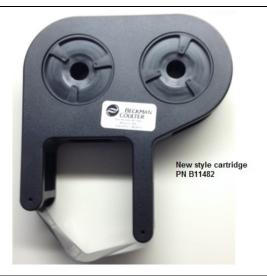
2 Ribbon must be between the plastic cartridge cover and metal rollers
